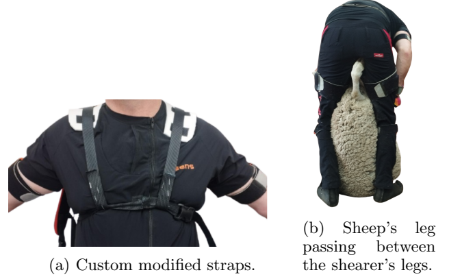
Figure 3: Possible interferences with the exoskeleton were identified for sheep shearing, a) shows how straps were modified and b) shows a possible incompatibility with the original device and the shearing task.
