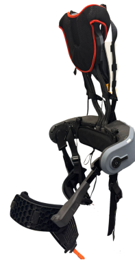
Figure 2: The FIT-HV lumbar exoskeleton with hardware modifications used in this study.
